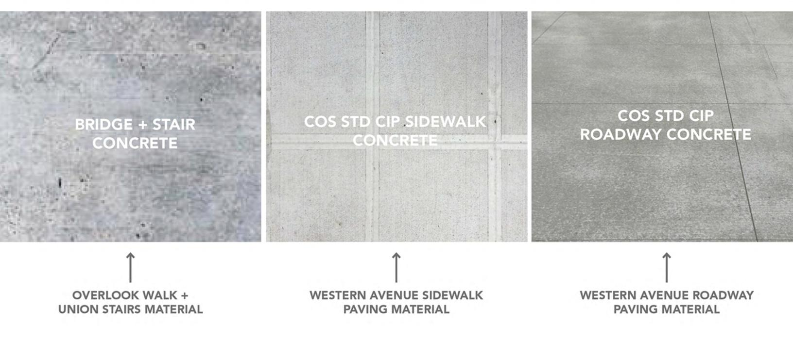
COS STANDARD ROADWAY CONCRETE (DARKENED) MAIN CORRIDOR SMALL EXP AGGREGATE CONCRETE UNION STREET PEDESTRIAN BRIDGE 90% DESIGN COS STANDARD PAVING SURFACES AT LOWER LEVEL **CURB RAMPS EXISTING CROSS-SECTION** - ALASKAN UNION STREET WAY SEATTLE ANTIQUES MARKET **EXISTING** COS STANDARD -**CURB RAMPS** COS STANDARD 1 1 **ROADWAY CONCRETE** (DARKENED) 1 1 COS STANDARD ROADWAY SMALL EXPOSED AGGREGATE CONCRETE (DARKENED) CONCRETE EXISTING PUBLIC STORAGE PLAN
