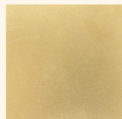
MTL1 Naval Brass C464 (60% Copper, 40% Zinc) Door cladding and fins
