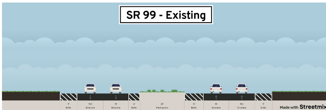
Figure 18: Existing SR 99 cross section
