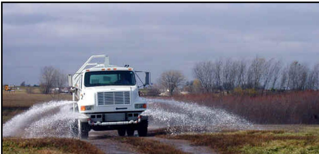
Figure 11. Using a Water Truck for Dust Control.
