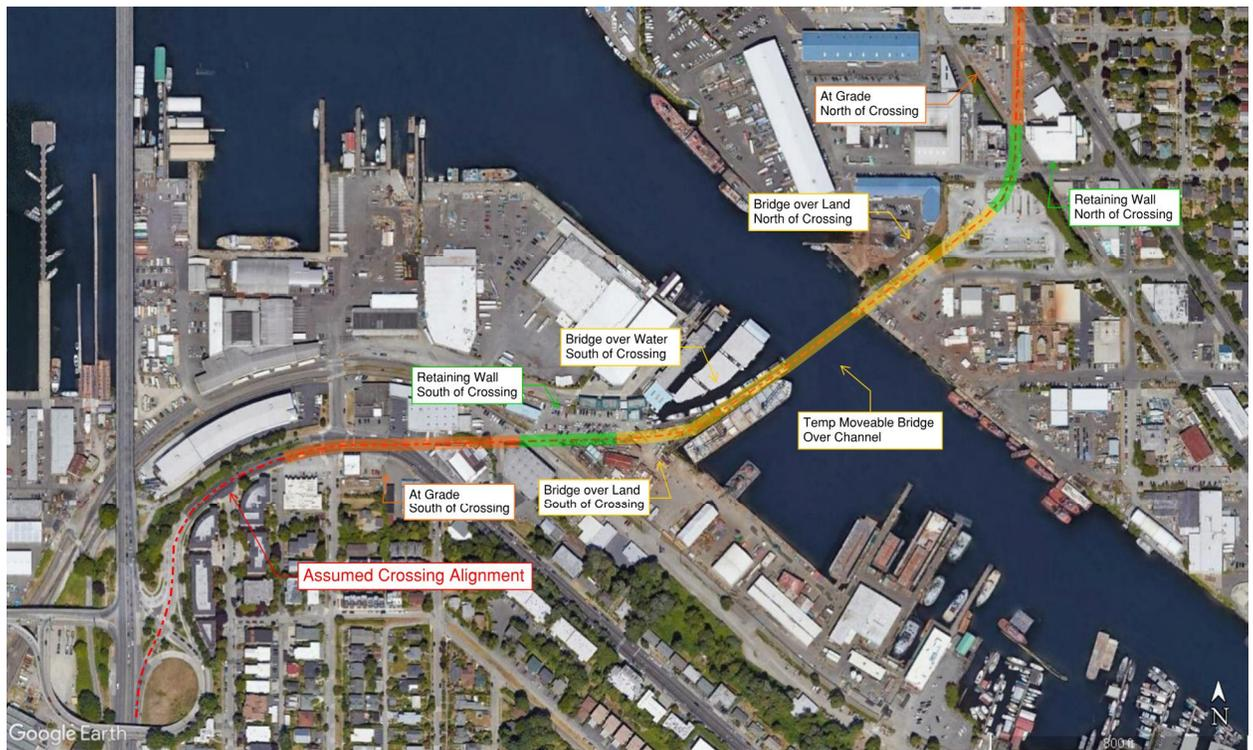
Figure 3.2 Temporary Detour Bridge Concept
