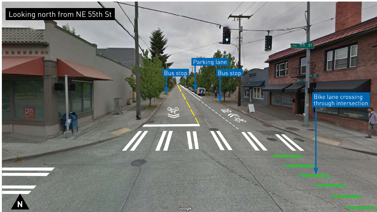
Conceptual design of 35th Ave NE between NE 47th St and NE 65th St; image not to scale
