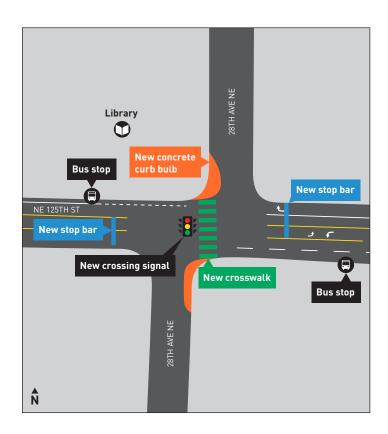
Note the addition of a new curb bulbs on the northwest & southeast corner of 28th and 125th. This adds to the safety of the intersection by shortening the crossing distance and increasing the visibility of people waiting to cross the intersection.
