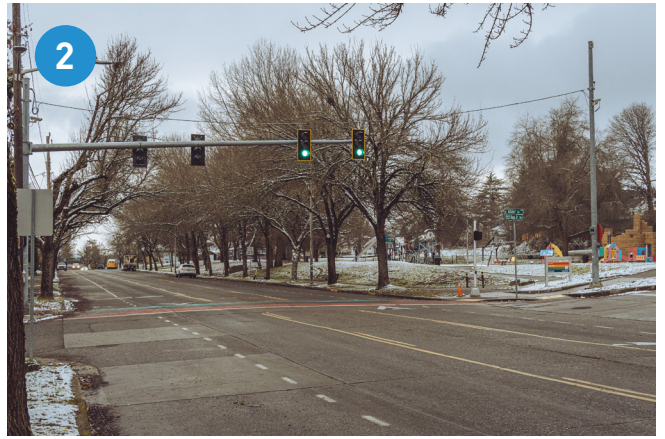
Pedestrian half signal at MLK Jr Way and E Alder St
