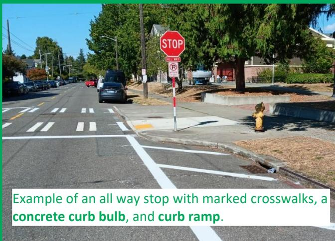
Example of an all way stop with marked crosswalks, a concrete curb bulb, and curb ramp.
