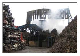
Figure 5: Metal shredder<sup>2</sup>.
